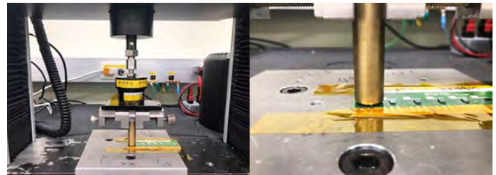
Figure 44: Pressure test instrument. The tester head lowers to the backside of the devices using a constant loading speed of 0.6 mm/min until the predetermined force is sensed by the gauge. The DUTs are surface mounted on a FR4 test coupon that is secured on the testing stage.
